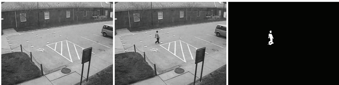
Fig. 1. Background subtraction results for the static unimodal Gaussian model. Left: static background image. Middle: image with human. Right: background subtraction results using the method in (2.4)
