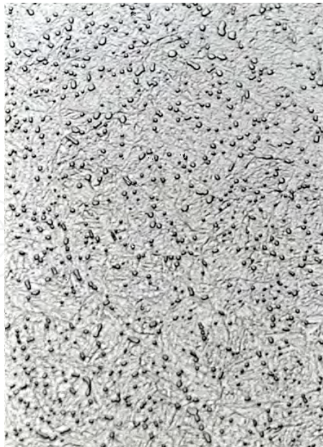
Fig. 5. Tempered microstructure of a nitrogen alloy martensite (1.4108). (M 1000:1)
