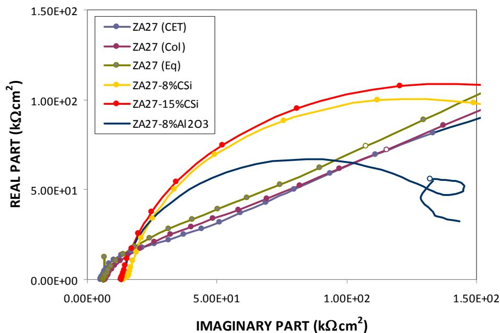
Fig. 6. (a) Nyquist Diagram for different samples.
