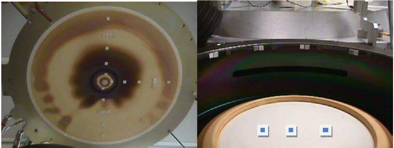
Fig. 9. Test coupons in etching chamber are mounted on chamber top window (left) and on chamber wall (right) and on the dummy aluminum wafer on an electrostatic chuck surface (right, white surface).
