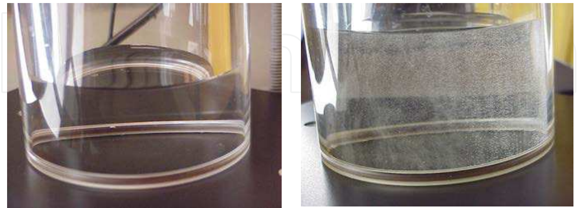
Fig. 24. Acidic corrosion resistance of two test coupons of anodized aluminum. On the left, anodized aluminum does not show any acidic corrosion in two hours and on the right, anodized aluminum shows severe acidic corrosion after only 10 minutes immersion in the acid.
