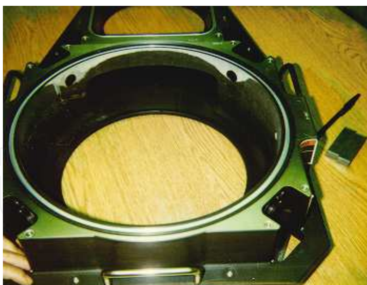
Fig. 5. Anodized aluminum is fully removed under \text{Cl}_2/\text{BCl}_3 plasma after only 1,800 wafers in production (about 60 RF hours). The special attacking pattern depends on the local plasma density and gas concentration.
