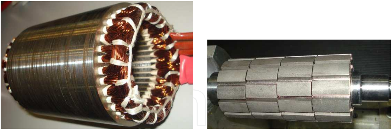
Fig. 5. Stator stack showing the motor laminations
