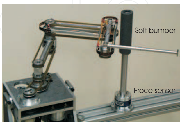
Fig. 13. Experimental manipulator with external force sensor
