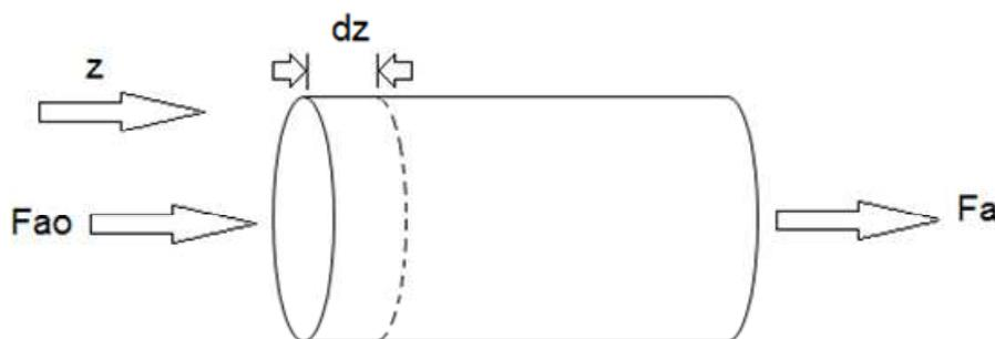
Fig. 2.2.1. Reactor differential volume representation.
