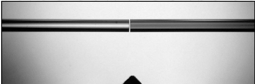
Fig. 24. SMF (left) and PCF (right) cleaved and positioned before fusion.
