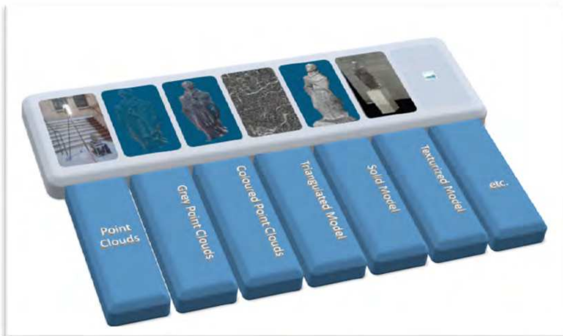
Fig. 21. Process products and stages of a laser scanner modelling project.
