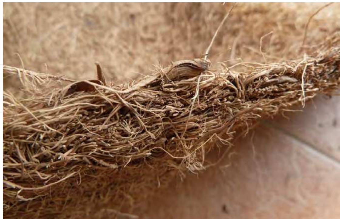
Fig. 10. Longitudinal cross section of OPEFB sheet
