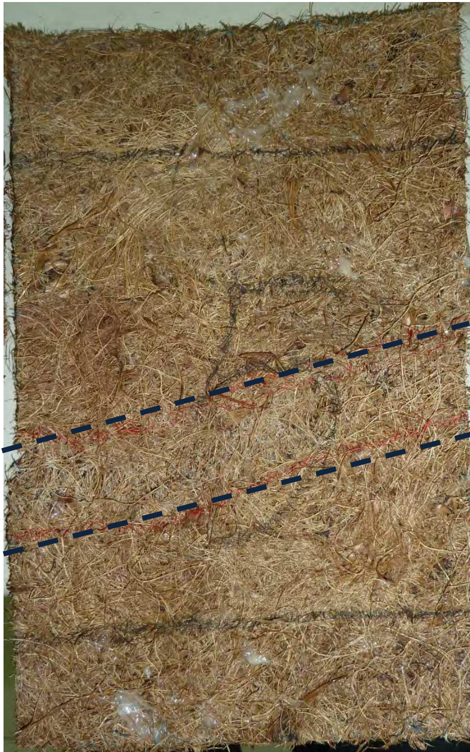
Fig. 13. Rupture area for 5% ABS coated OPEFB sheet
