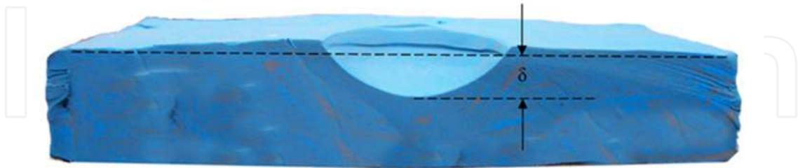
Fig. 20. Impact depth of witness material: commercial plastilene Modelina
