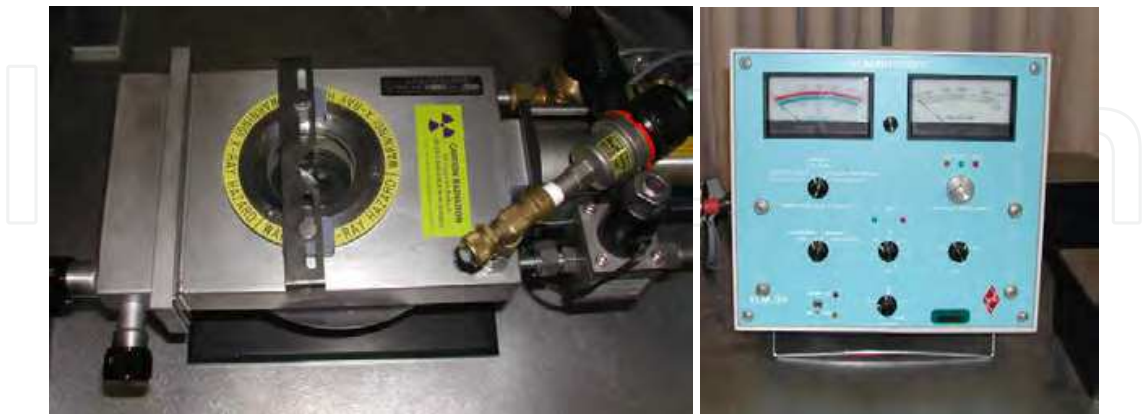
Fig. 2.4. Left: Luminoscope sample holder. Right: Luminoscope control and electronics.
