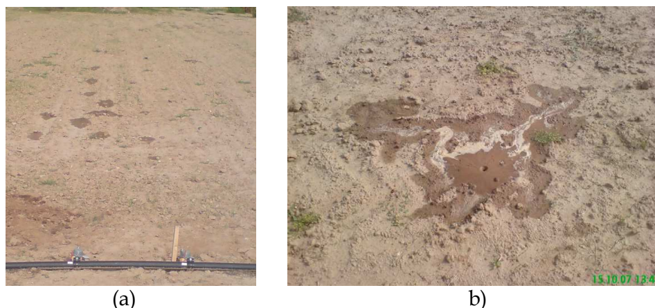
Fig. 5. Surfacing in SDI units: (a) wetted soil surface above the laterals and (b) detail of the wetted area.
