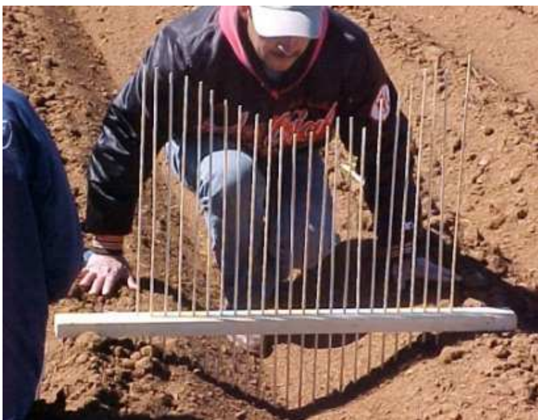
Picture 1. Furrow profilometer for determining cross-sectional area
