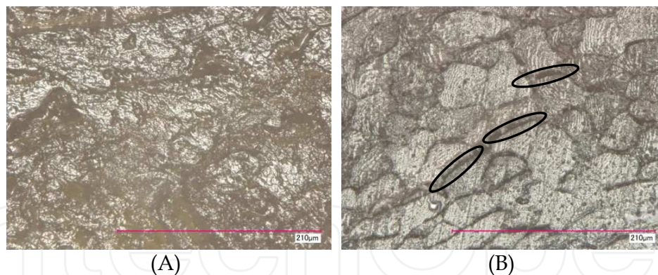
Fig. 22. Optical microscope photographs ( \times 1000 ) of the cross-section for P_H , (A): 127%-d.b., (b): 54%-d.b.
