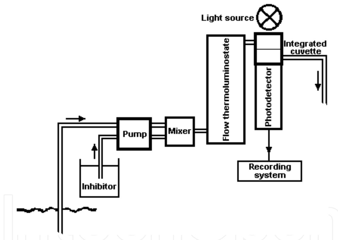
Fig. 6. Schematic diagram of flow luminometer for *on line* registration of delayed luminescence intensity of phytoplankton incubated in predefined temperature and light with and without electron transport inhibitor.
