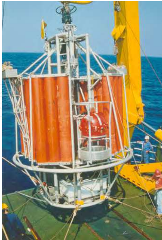
Fig. 3. NADIA observatory developed by Ifremer in 1985, © Ifremer
