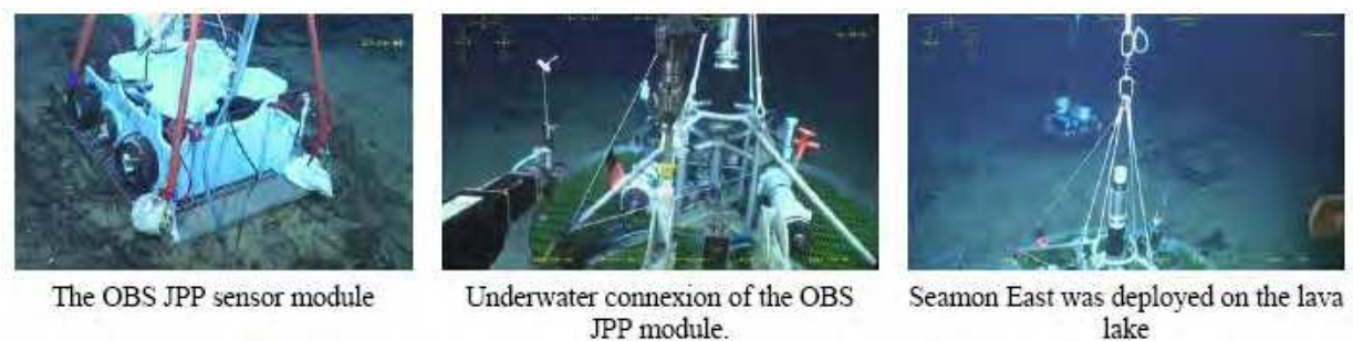
Fig. 16. Deployment and connection of the SEAMON East node, (lave Lake) © Ifremer/Victor 6000
