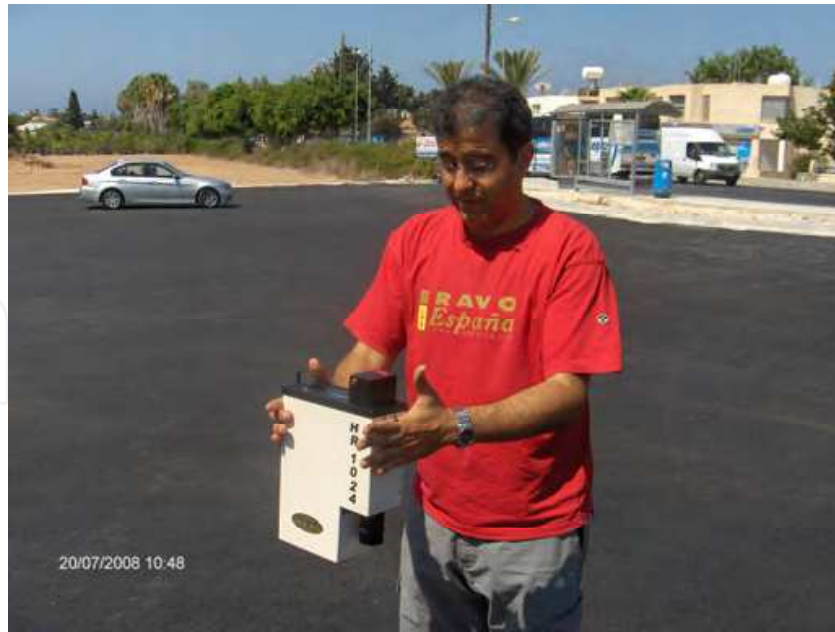
Fig. 10. Field spectroradiometric measurements over dark asphalt target.
