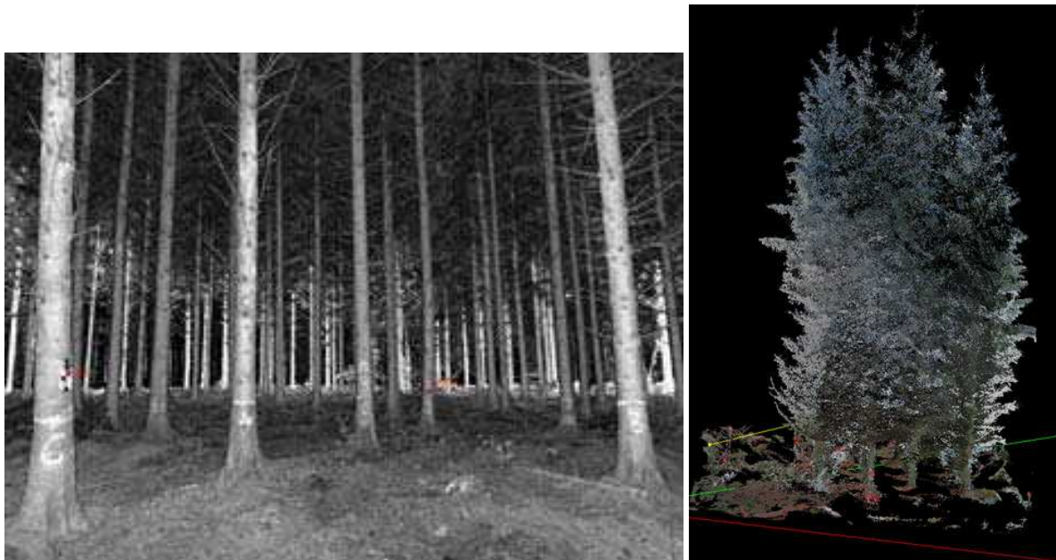
Fig. 7. Below-canopy plot sampling using terrestrial laser scanning. Images courtesy of Forest Research, UK.
