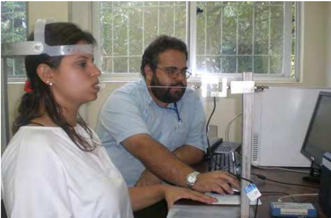
Fig. 7. Portable device for measuring the force of the lips: FORLAB.
