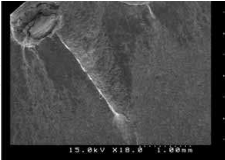
Fig. 43. Fatigue propagation area
