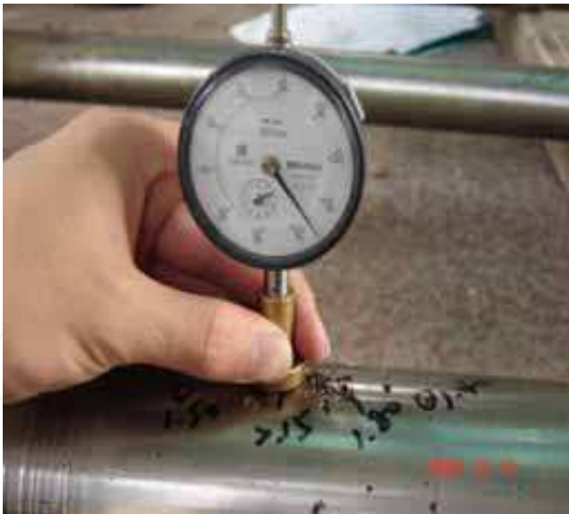
Fig. 2. Measuring depth of pitting deep
