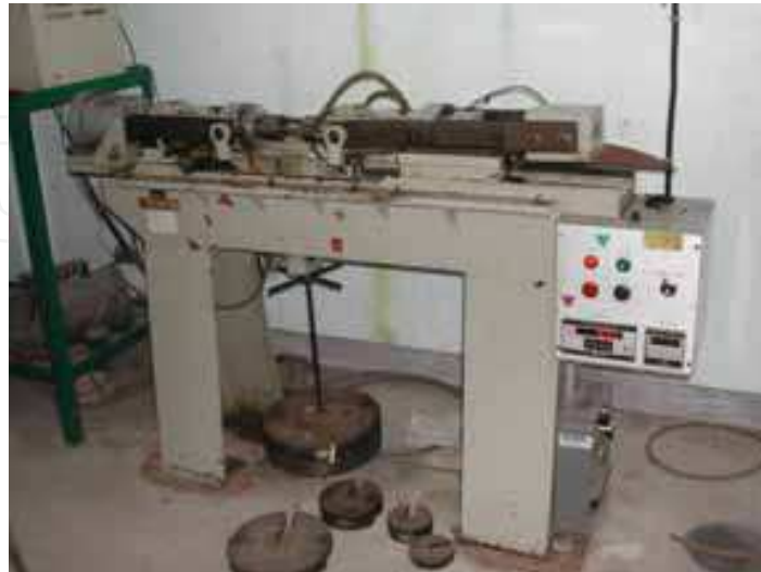
Fig. 39. Rotating bending fatigue test machine
