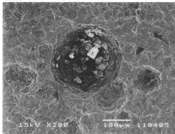
Fig. 7. Pitting corrosion in the specimen
