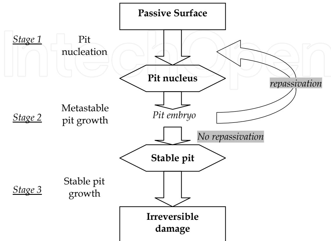
Fig. 4. Multistep mechanism for the onset of a stable pit (Jirarungsatian& Prateepasen, 2010)
