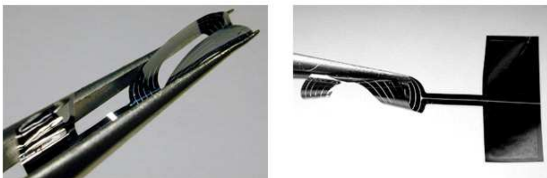
Fig. 7. Demonstration of the coil's flexibility and foldability. (Li et al., @ 2005 IEEE)
