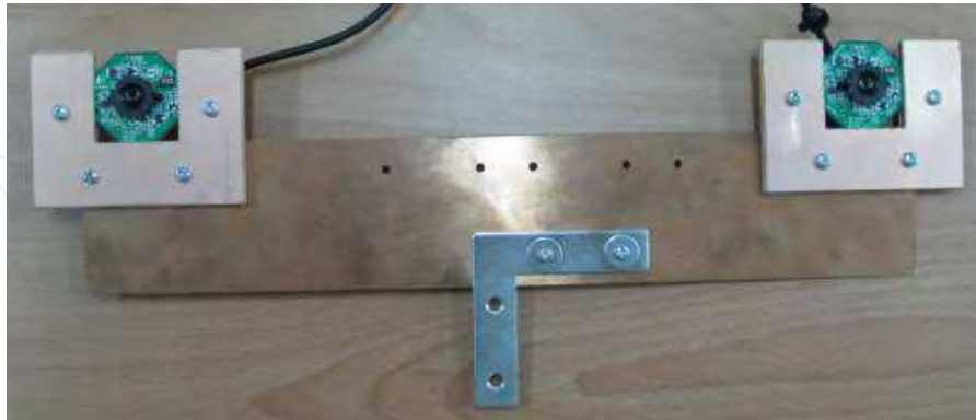
Fig. 1. The stereo vision system composed of two Logitech® webcams
