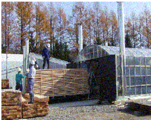
Photo 1. A Fully Passive Solar Lumber Drying House Loading Larch Lumber (2x4 material); (South-North model)
