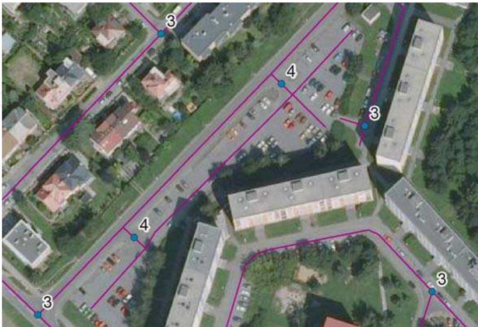
Fig. 4. Example of the merge intersection with Valence 4
