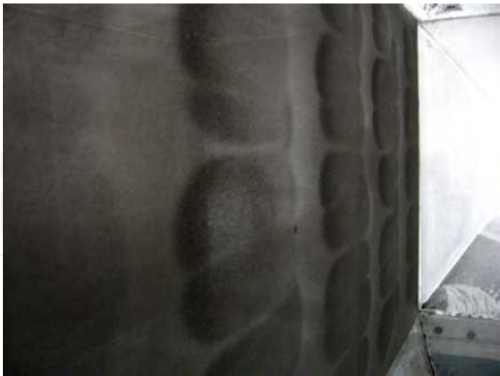
Fig. 23. Pattern of collected fly ash on CE electrodes for RDE-3 electrode.
