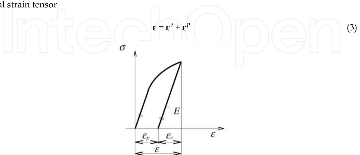
Fig. 10. Decomposition of total strain under uniaxial loading.
