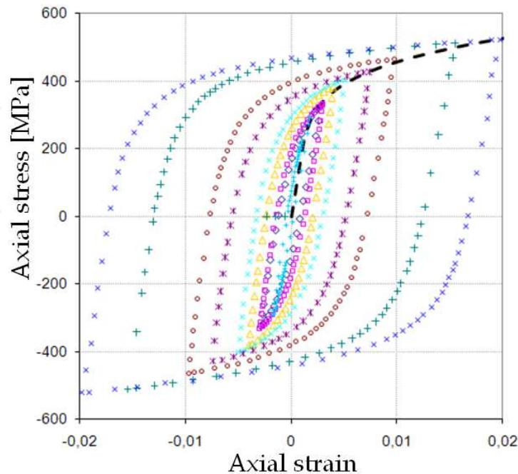
Fig. 3. Cyclic stress-strain curve of ST52 steel.
