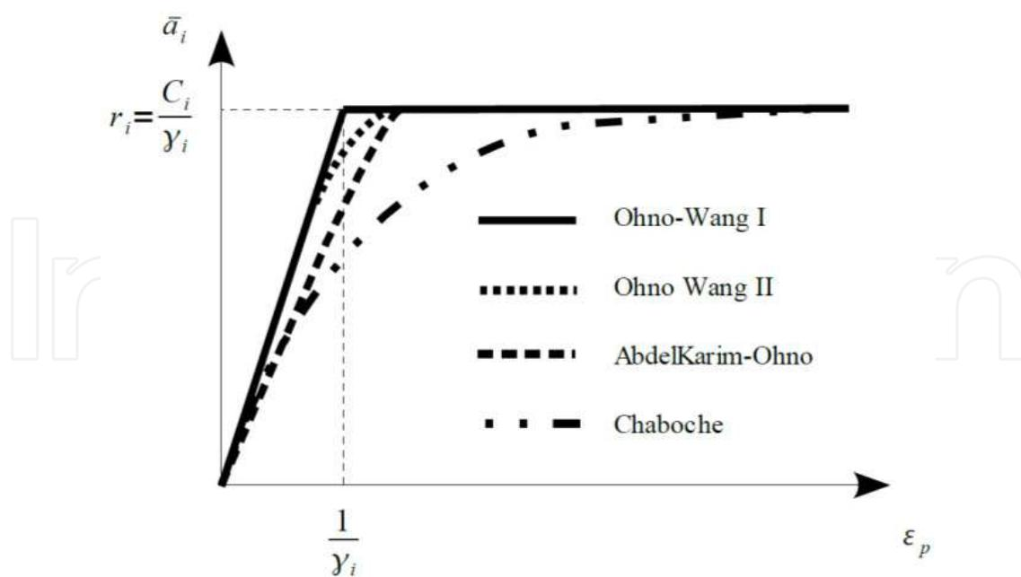
Fig. 18. Nonlinearity introduced in four basic cyclic plasticity models.
