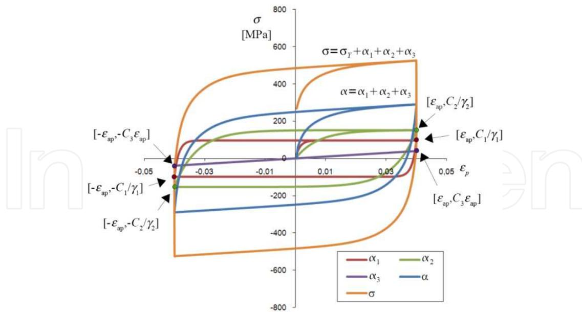
Fig. 15. Scheme for use of the hysteresis loop to identify parameters of Chaboche model.
