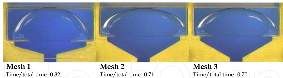
Fig. 10. Comparison of the effect of distributor geometry on the time it takes to reach the wall farthest from the injection port in a horizontal orientation.
