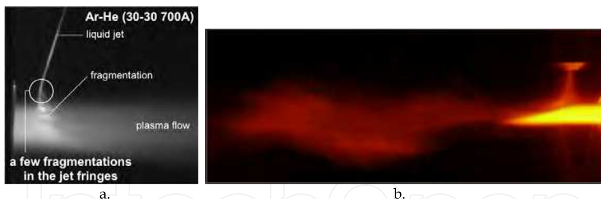
Fig. 5. (a) Example of fragmentation of an ethanol jet, about 300 \mu\text{m} in diameter, starting in the fringes of a d.c. plasma jet (Ar-He: 30-30 slm, 700 A, 40 V, Anode-nozzle i.d. 6 mm) Etchart-Salas et al (2007) , (b) Interaction of an Ar- \text{H}_2 plasma jet with atomized ethanol drops Fazilleau et al (2006) .
