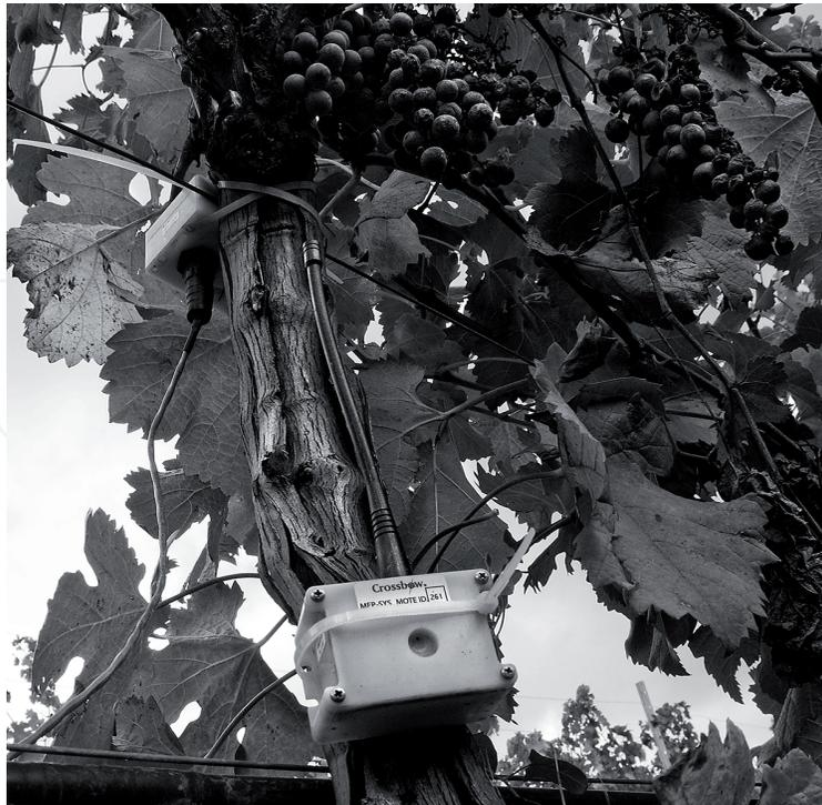
Fig. 2. WSN node attached to a vine in the Wisevine project.
