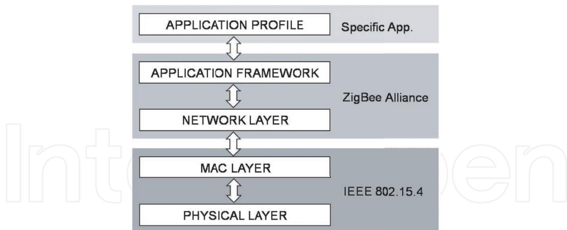
Fig. 3. ZigBee protocol stack.
