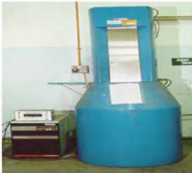
Fig. 6. \gamma -irradiation system model (J. L. Sherperd) at the Malaysian Nuclear Agency, Bangi - Malaysia UPM
