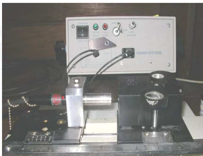
Fig. 4. Raman system and its accessories for sample set up and characterization, Faculty of Science, department of Physics - UPM
