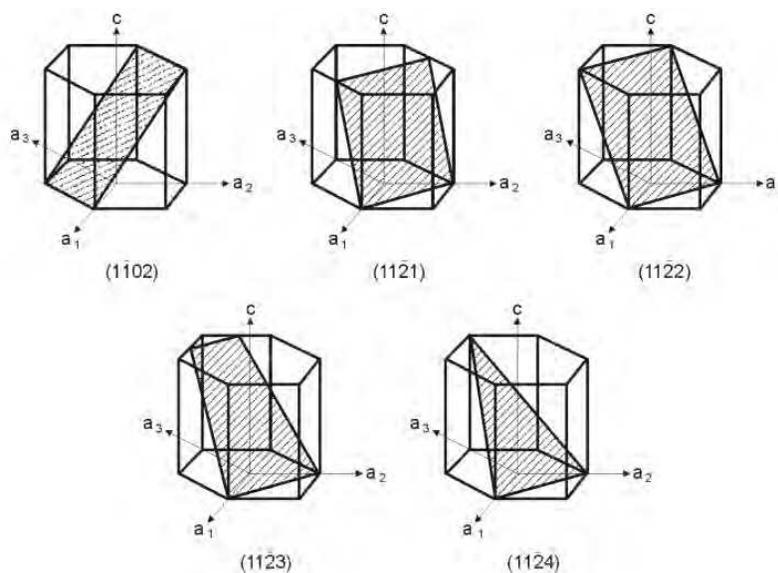
Fig. 3. Twinning planes in  $\alpha$  titanium (Balasubramanian & Anand, 2002)
