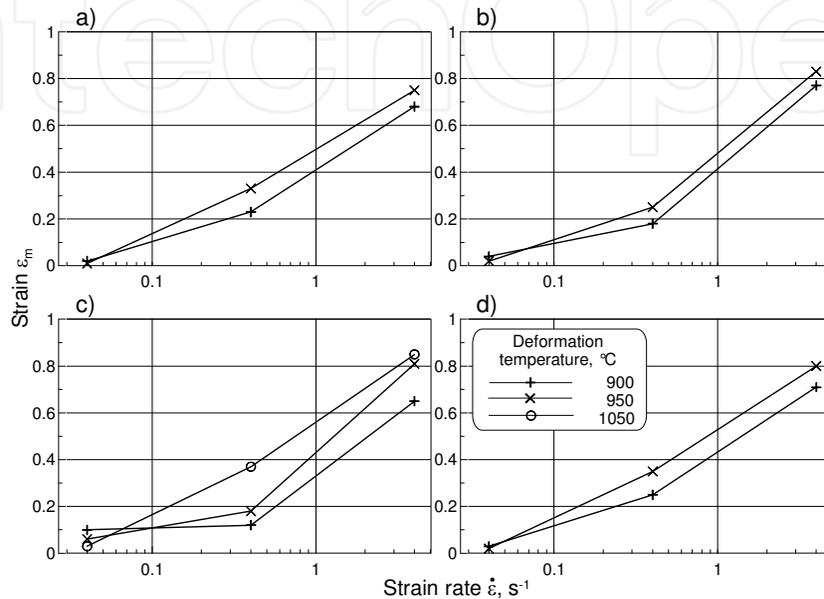
Fig. 27. The dependence of  $\epsilon_m$  strain on strain rate, temperature of deformation and microstructure of Ti-6Al-4V alloy: a) bi-modal, b) globular, c) coarse-grained lamellar, d) fine-grained lamellar microstructure (Kubiak, 2004)
