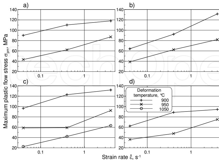
Fig. 28. The dependence of maximum plastic flow stress  $\sigma_{pm}$  on strain rate, temperature of deformation and microstructure of Ti-6Al-4V alloy: a) bi-modal, b) globular, c) coarse-grained lamellar, d) fine-grained lamellar microstructure (Kubiak, 2004)
