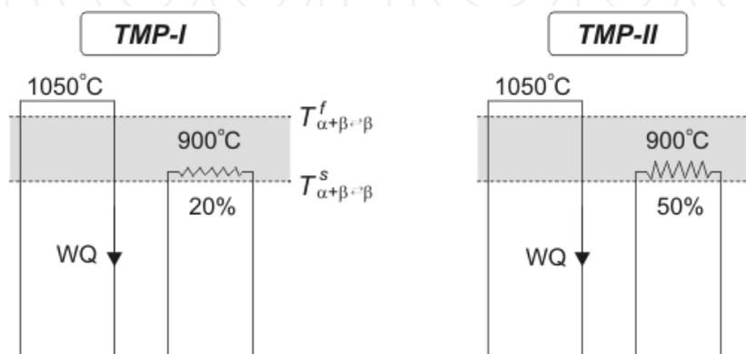
Fig. 29. Schemes of thermomechanical processing of Ti-6Al-4V alloy with forging reduction  $\varepsilon \approx 20\%$  (a) and  $\varepsilon \approx 50\%$  (b) (WQ - water quenching) (Motyka & Sieniawski, 2010)
