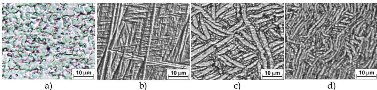
Fig. 30. Microstructure (DIC) of Ti-6Al-4V alloy before thermomechanical processing (a), after quenching from the  $\beta$  phase range (b) and after deformation in the  $\alpha+\beta \leftrightarrow \beta$  range with forging reduction of 20% (c) and 50% (d) (Motyka & Sieniawski, 2010)
