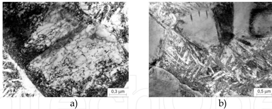
Fig. 35. Microstructure (TEM) of Ti-6Al-2Mo-2Cr alloy after TMP-II process: dislocations in  $\alpha$  grains (a), precipitations of  $\alpha$  grains in  $\beta$  transformed phase (b) (Motyka & Sieniawski, 2010)
