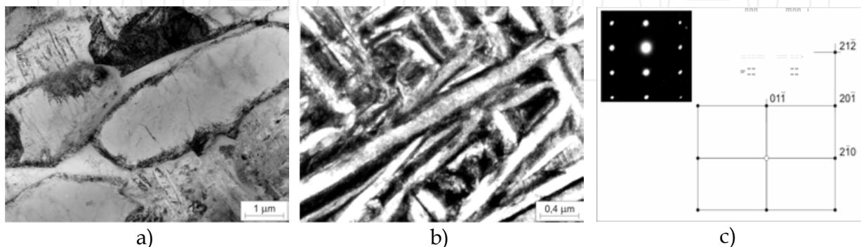
Fig. 34. Microstructure (TEM) of Ti-6Al-2Mo-2Cr alloy after TMP-II process: dislocations in  $\alpha$  grains (a), lamellae precipitations of  $\alpha$  grains in  $\beta$  transformed phase (b) with indexing of diffraction (c) (Motyka & Sieniawski, 2010)
