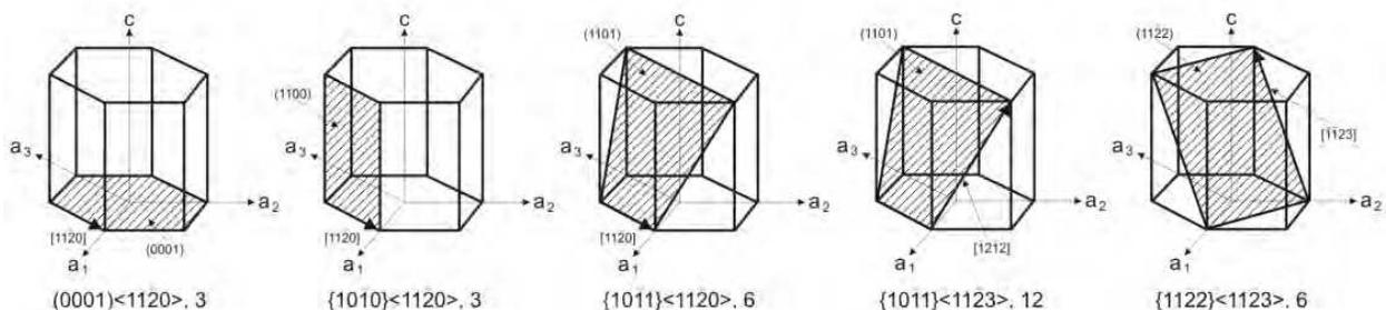
Fig. 1. Slip systems in  $\alpha$  titanium (Balasubramanian & Anand, 2002)
