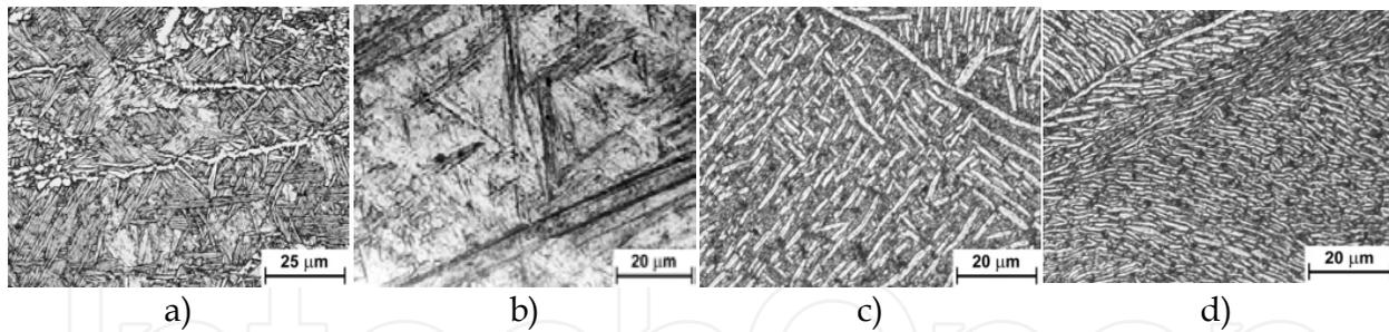
Fig. 31. Microstructure (DIC) of Ti-6Al-2Mo-2Cr alloy before thermomechanical processing (a), after quenching from the  $\beta$  phase range (b) and after deformation in the  $\alpha+\beta\leftrightarrow\beta$  range with forging reduction of 20% (c) and 50% (d) (Motyka & Sieniawski, 2010)
