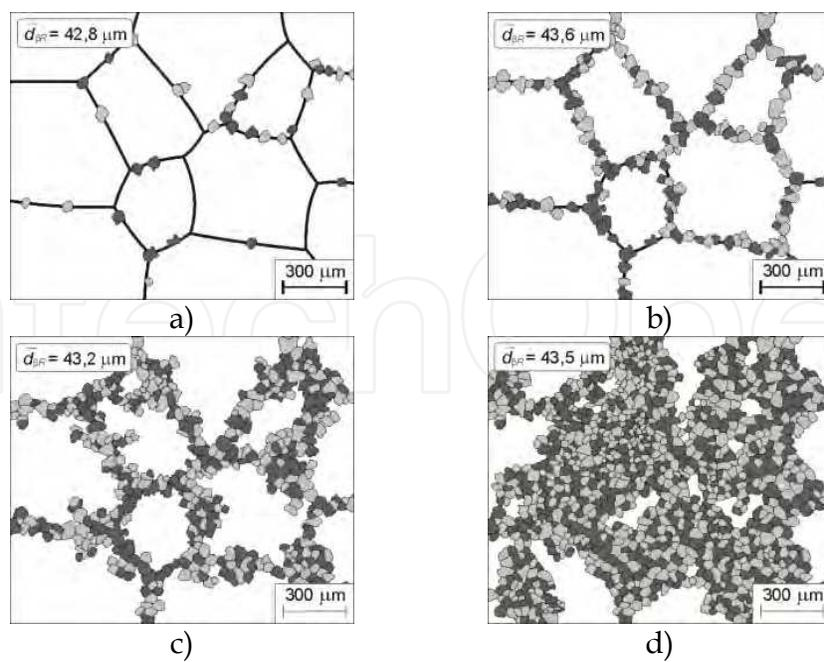
Fig. 20. Simulation of microstructure development for Ti-6Al-4V alloy deformed at 1050°C at the strain rate  $\dot{\epsilon} = 1.0 \text{ s}^{-1}$  for various strains: a)  $\epsilon = 0.7$ ; b)  $\epsilon = 5.0$ ; c)  $\epsilon = 15$ , d)  $\epsilon = 45$ ;  $\bar{d}_{\beta R}$  - average diameter of recrystallized  $\beta$  grains (Ding et al., 2002)
