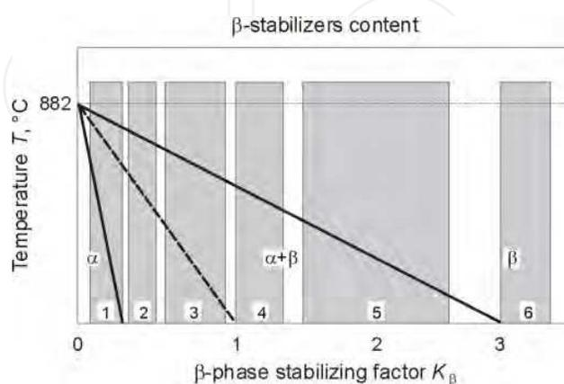
Fig. 4. Classification of titanium alloys on the basis of  $\beta$  stabilizers content: 1 –  $\alpha$  alloys, 2 – near  $\alpha$  alloys, 3 – martensitic  $\alpha+\beta$  alloys, 4 – transition  $\alpha+\beta$  alloys, 5 – near  $\beta$  alloys, 6 –  $\beta$  alloys (Glazunov & Kolachev, 1980)
