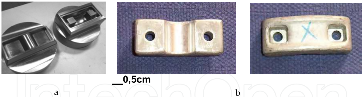
Fig. 15. (a) HPDC molds, and (b) resultant piece produced by MSC&HPDC.
