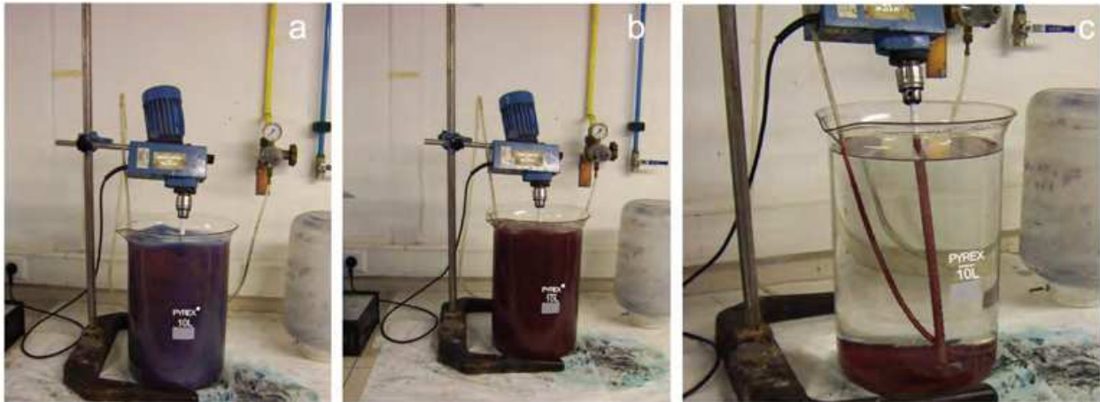
Fig. 4. Evolution of the plating bath, (a) 0 min, (b) 10 min and (c) 40 min.
