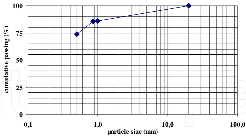
Fig. 24. Flexible multi-layered sachets, 20 mm grid, cumulative passing, dry comminution.
