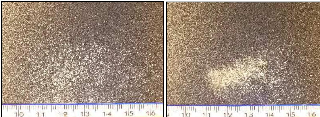
Fig. 11. Comminuted flexible multi-layered sachets containing granular medicine, belonging to the size class  $-0.5$  mm, obtained in the preliminary tests without control grid (left) and with 20 mm mesh control grid (right).
