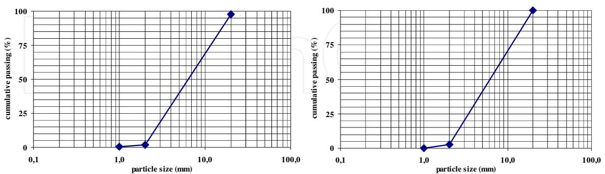
Fig. 19. Plastic bags and films, 20 mm grid, cumulative passing, dry (left) and wet (right) comminution.
