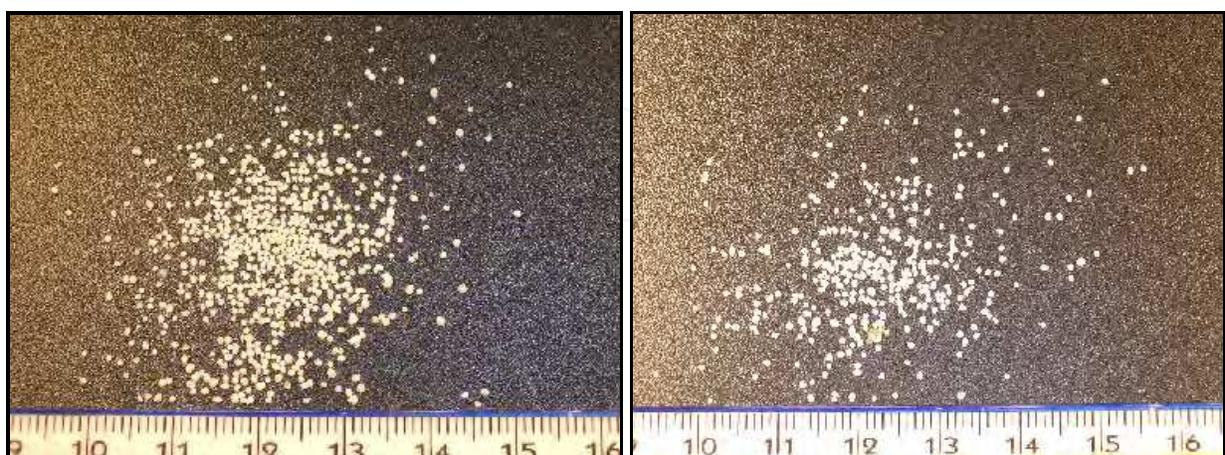
Fig. 10. Comminuted flexible multi-layered sachets containing granular medicine, belonging to the size class -1.0 +0.5 mm, obtained in the preliminary tests without control grid (left) and with 20 mm mesh control grid (right).
