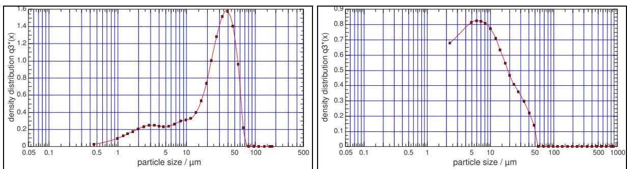
Fig. 17. Bottles in PET, 20 mm grid, size distribution, dry comminution, size class  $+2.0 - 1.0 \text{ mm}$  (left) and  $-1 \text{ mm} +38 \mu\text{m}$  (right), laser granulometry.
