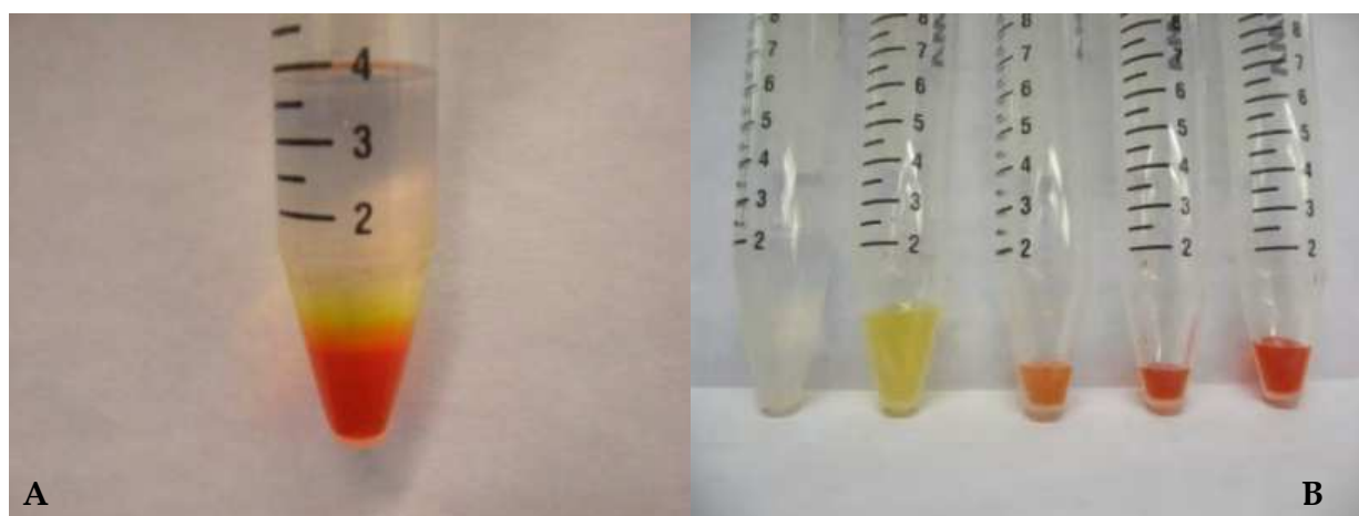
Fig. 10. (A) The separation of a CdTe NC dispersion (with size range in the 3-5 nm range) into different precipitation bands following centrifugation. (B) The separation of the bands into different vials through pipetting.
