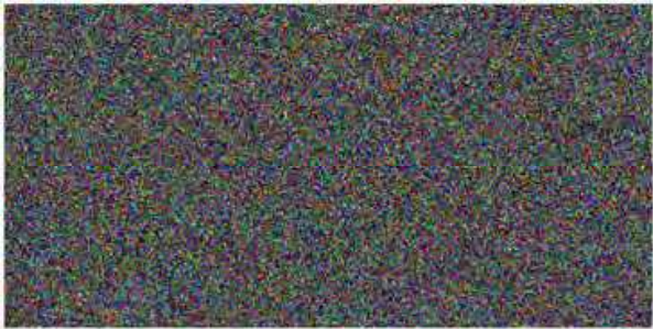
Fig. 19. The difference between the ciphertexts A and B. The initial 20000 samples of random sequences, generated with a model of the Chua's Circuit, were left out.
