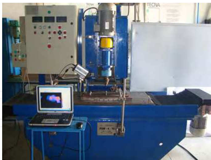
Fig. 22. FSW machine from ISIM Timișoara, Romania
