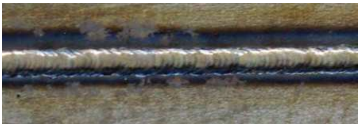
Fig. 20. Welded bead visual aspect for LASER-TIG variant
