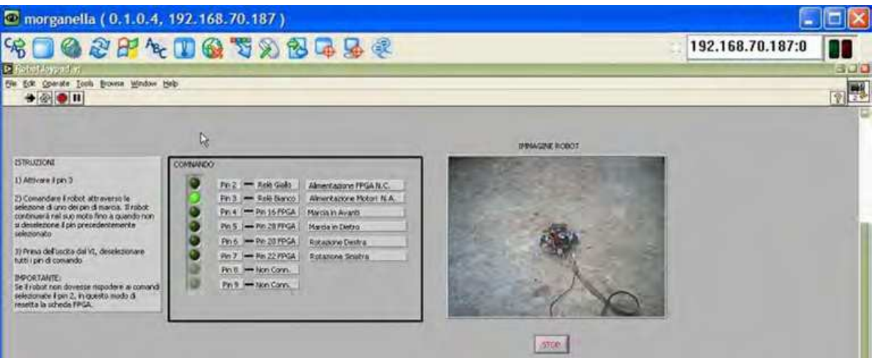
Fig. 11. VI front panel of the two-wheel vehicle.
