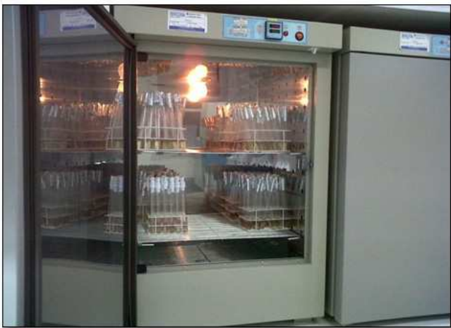
Fig. 6. Samples of packaging positioned from 0 to 5 for EtO penetration analysis.
