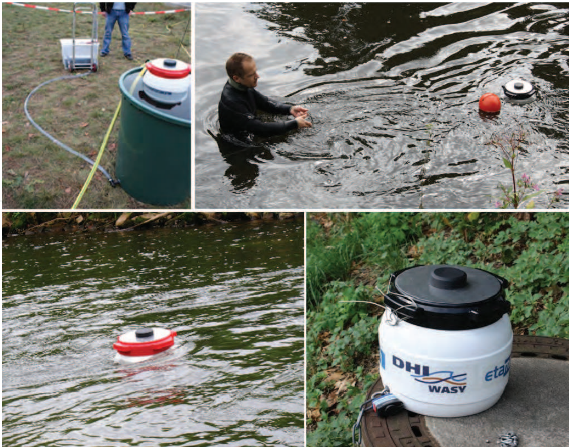
Fig. 2. Deployment of a G-WaLe floater in a river.
