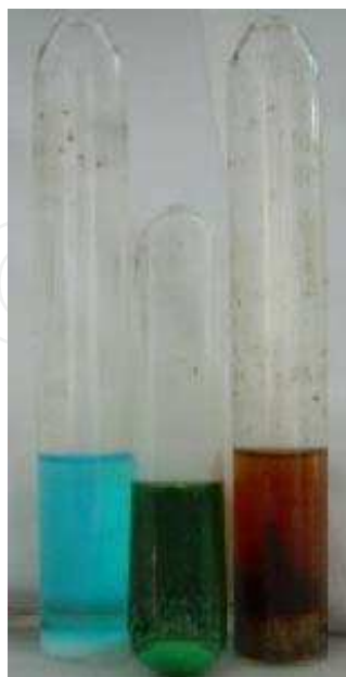
Fig. 13. Digital photograph showing various stages of the hydrothermal reduction of reaction of \text{Cu}_2\text{O} in a sealed tube.
