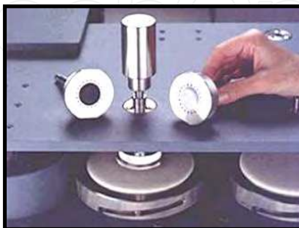
Fig. 16. Setting of sock kit on Martindale apparatus
