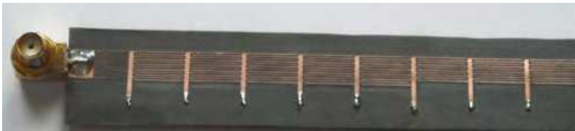
Fig. 43. A prototype and its detail of Radiation patter of tapered 16 unit-cell CRLH-TL LWA made on Rogers RT/duroid 5880.
