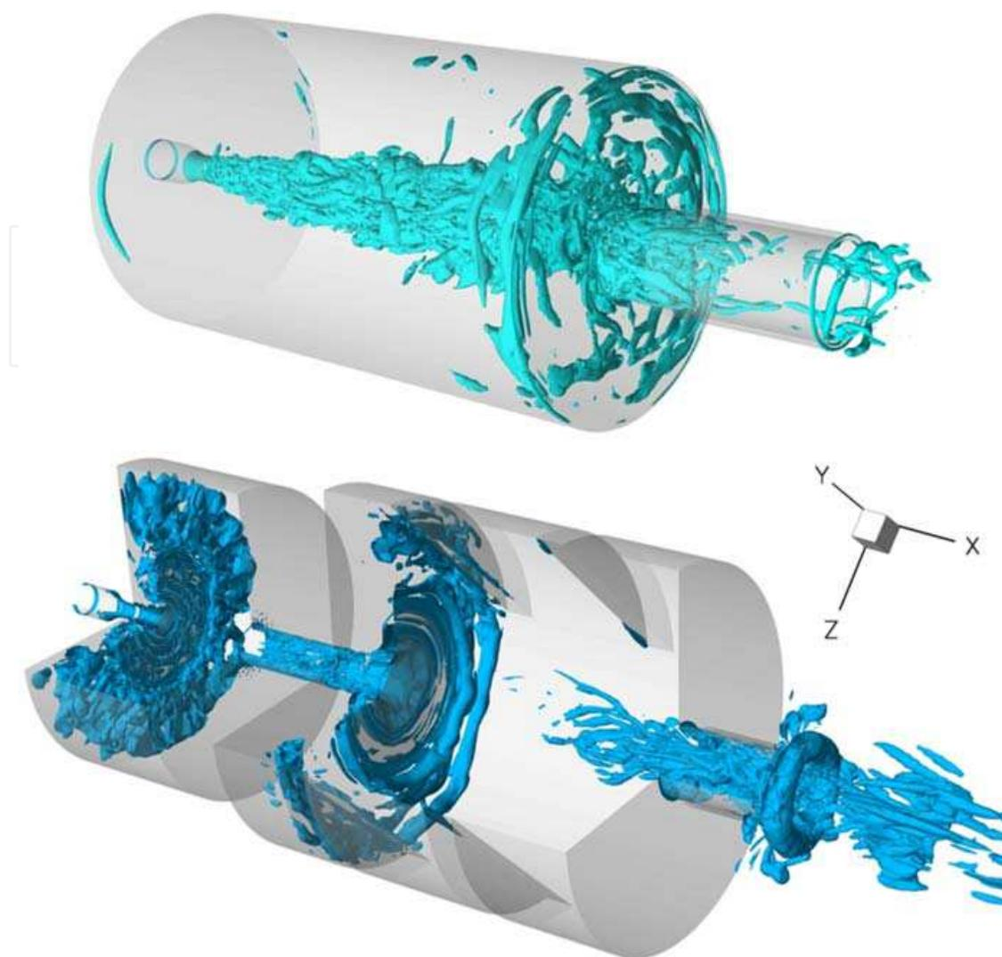
Fig. 9. Flow pattern in the resonators: iso-surfaces of the  $Q$ -criterion at  $5 \cdot 10^4 \text{ s}^{-2}$  in the single resonator (top) and at  $10^4 \text{ s}^{-2}$  in the coupled resonators (bottom)
