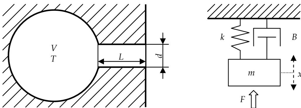
Fig. 2. The Helmholtz resonator and a mass-spring-damper system
