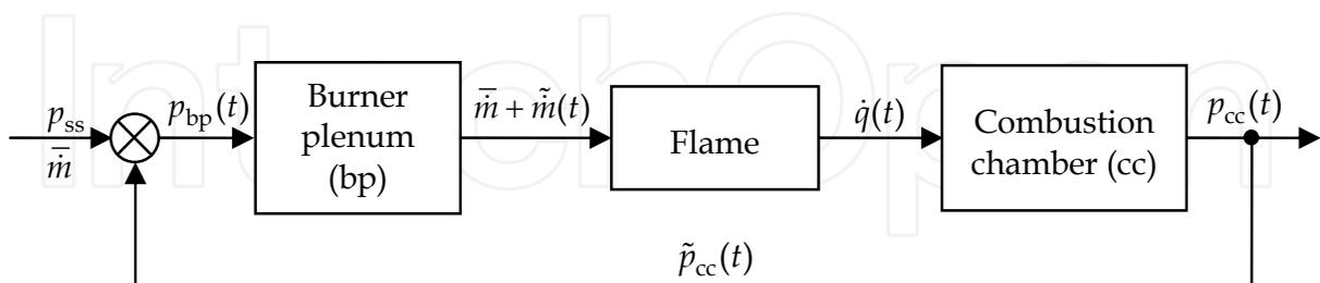
Fig. 1. Feedback loop of a combustion system with mass flow rate, pressure and heat release rate signals
