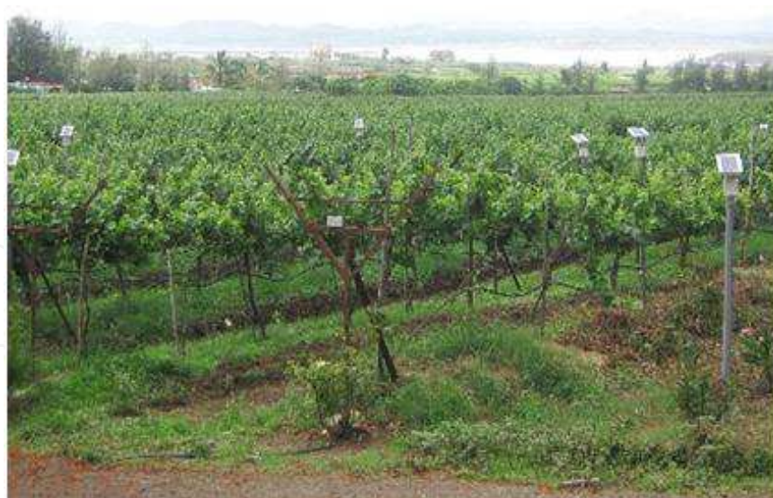
Fig. 2.3. Wireless Sensor Network Deployment at Vineyard, Nashik, MH, India
