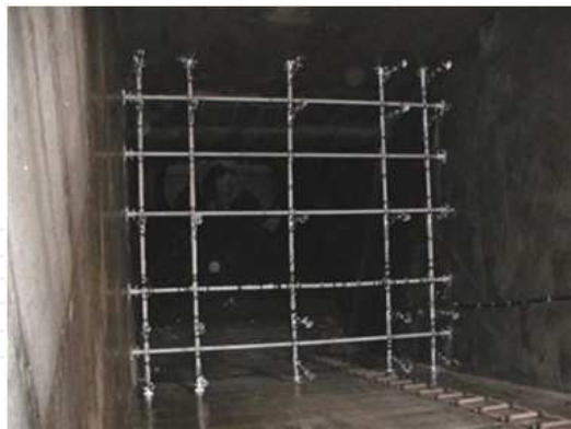
Fig. 14. Hydrometric section with the supporting frame and installed current-meters (own application).
