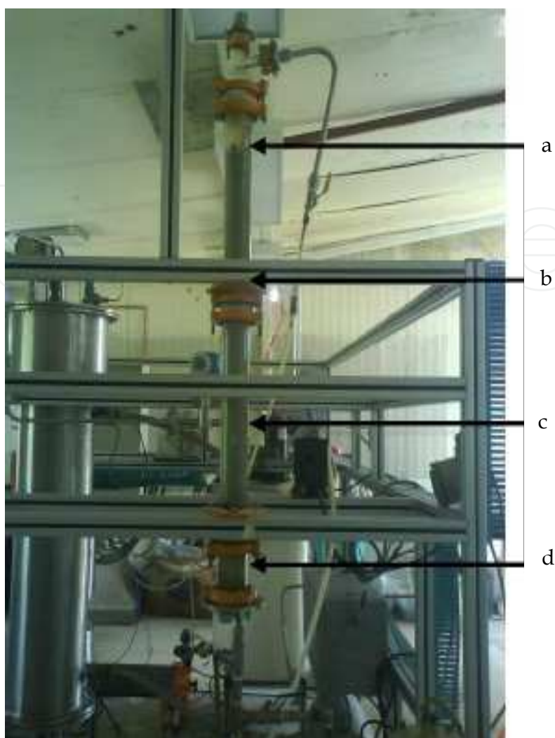
Fig. 3. Biofiltration system coupled to an anaerobic digestion system. Arrows indicate the position of sampling used for DGGE analysis.
