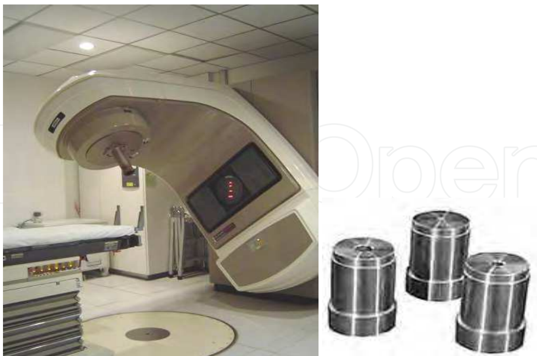
Fig. 11. Linac-based radiosurgery machine and circular collimators
