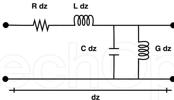
Fig. 2. Transmission line model per unit length  $dz$ .
