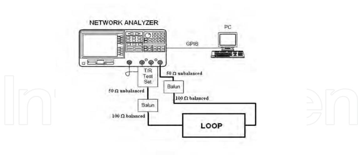
Fig. 6. Experimental setup used during the measurements campaign.
