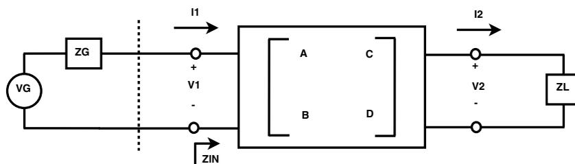
Fig. 3. Two-port network model.
